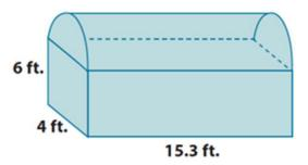
The rectangular prism at the bottom has the following volume:  $V = 4 \times 15.3 \times 6 = 367.2.$
