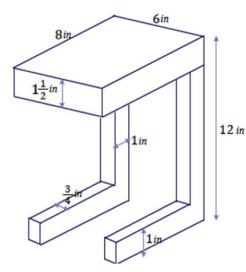
Volume of bottom $V = 2(8 \text{ in.} \cdot 1 \text{ in.} \cdot 0.75 \text{ in.})$ legs: $= 12 \text{ in}^3$ Volume of vertical $V = 2(1 \text{ in.} \cdot 9.5 \text{ in.} \cdot 0.75 \text{ in.})$ legs: $= 14.25 \text{ in}^3$ Volume of tabletop: $V = 8 \text{ in.} \cdot 6 \text{ in.} \cdot 1.5 \text{ in.}$  $= 72 \text{ in}^3$
