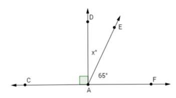
$\angle CAD$ ,  $\angle DAE$ , and  $\angle FAE$  are angles on a line and their measures sum to  $180^{\circ}$ .
